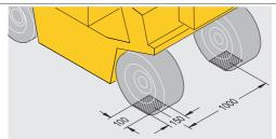
In the drawing measures for a leveler with a load capacity of 100kN or 150kN are shown.
