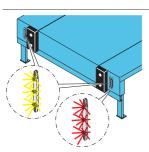
ASSA ABLOY Dock-IN offers a complete line of guide- and traffic lights that align the truck with the docking bay to make the dock-in procedure easy and safe. ASSA ABLOY Dock-IN is based on modern LED technology and stands for high reliability and low energy consumption.
