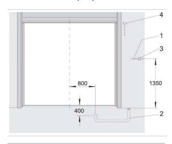
1 Mains supply: 3/N/PE AC 50 Hz
