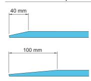
The standard steel lip is 40 mm bevelled. Optionally, the lip can be bevelled 100 mm, designed to provide maximum comfort and smooth transition from the lip.
