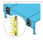
ASSA ABLOY Dock-IN White consists of two white LED light bars. It is designed to help guide a truck to the dock. ASSA ABLOY Dock-IN White offers much more visual aid than white stripes on the shelter or asphalt. Mounted on the wall they are always clearly visible, less exposed to wear and tear and not hidden by dirt and snow!
