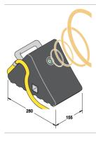
The wheel chock has a sensor to detect the presence and position of the vehicle and is connected to the dock leveler control panel. If no vehicle is detected, the docking station is blocked for safety reasons. Furthermore, the wheel chock prevents the vehicle from moving during loading/unloading.
