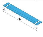
Ensures that the swing lip reaches the lorry bed by folding down one or both outer segments when the lorry is smaller than usual, or not parked in the exact centre position. Avoids damage to the truck and interruption of the dock-in procedure. Only available for 60 kN. Z = 125 mm
