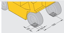
In the drawing measures for a leveler with a load capacity of 100kN or 150kN are shown.
