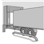
This visual aid makes it easier to park the vehicle and reduces the risk of collision. Especially advantageous for docking stations with wide leveler lips and cushion shelters. Parking guides can be bolted or cast in concrete on the floor before the leveler.
