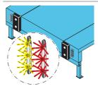
ASSA ABLOY Dock-IN White & Red is the optimum combination of both systems for easy and safe docking. The white LEDs provide the visual target and the red LED positions the truck at the right distance to the dock. The white guiding LEDs turn off when the truck is detected and at the same time the red LED turns ON. ASSA ABLOY Dock-IN White & Red guide the truck driver in the best possible way for an easy and safe docking.
