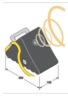
The wheel chock has a sensor to detect the presence and position of the vehicle and is connected to the dock leveler control panel. If no vehicle is detected, the docking station is blocked for safety reasons. Furthermore, the wheel chock prevents the vehicle from moving during loading/unloading.
