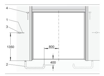
1 Mains supply: 3/N/PE AC 50 Hz 400V 3-phase, 230V 3-
