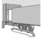
This visual aid makes it easier to park the vehicle and reduces the risk of collision. Especially advantageous for docking stations with wide leveler lips and cushion shelters. Parking guides can be bolted or cast in concrete on the floor before the leveler.
