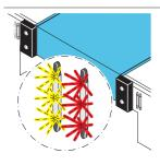
ASSA ABLOY Dock-IN White & Red is the optimum combination of both systems for easy and safe docking. The white LEDs provide the visual target and the red LED positions the truck at the right distance to the dock. The white guiding LEDs turn off when the truck is detected and at the same time the red LED turns ON. When the truck is leaving the white LEDs turn ON. ASSA ABLOY Dock-IN White & Red guide the truck driver in the best possible way for an easy and safe docking.
