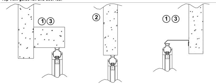
Installation surfaces for the header box must be flat, parallel and deviate maximum 5 mm from a horizontal line.
