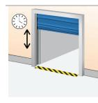
A programmable timer that closes the door after a specified time, counted from either the fully open position and/or from passing the photocell beam. A sensor, e.g. a magnetic loop or a radar, is used for automatic opening.
