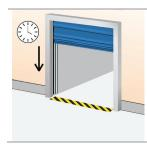
A programmable timer that closes the door after a specified time, counted from either the fully open position and/or from passing through the photocell beam. Selector switch in control unit.
