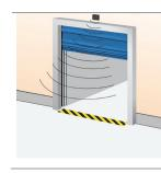
An infrared sensor above the door detects an object (person, vehicle) within a specified distance from the door and opens the door automatically. This is an ideal solution for frequent vehicle or personal traffic. Often combined with automatic closing. Installed on the inside or outside wall above the door.
