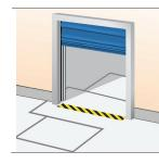
A sensor in the floor detects a metal object (usually forklift trucks, pallet trucks) and opens the door automatically. This is an ideal solution for frequent vehicle traffic. Installed on the outside, inside or both sides of the door in the ground.
