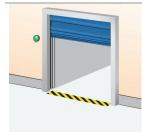
One or two green warning lights indicating the open position of the door by continuous light signal. Installed on the inside and/or outside wall beside the door.
