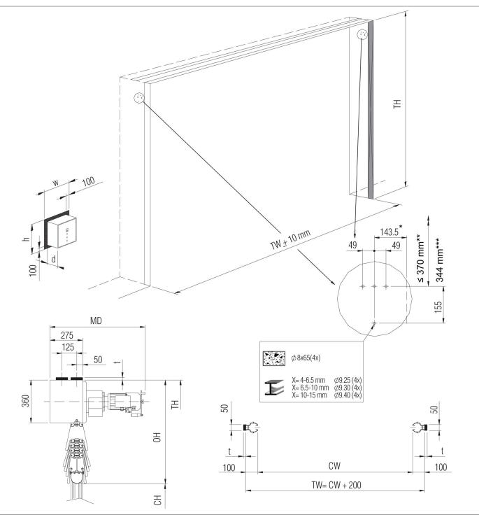
The S800 vertical fabric folding door can also be provided with a self-supporting header box. The upper fixing surfaces are then replaced by surfaces for securing brackets.
