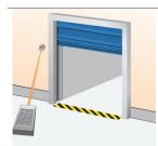
A hand-held radio transmitter allows door operation from a vehicle or any position within 50-100 meters from the receiver and aerial at the door.
