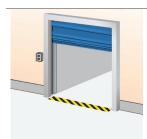
An extra control box is installed outside the building or inside close to the door if the main control unit needs to be installed away from the door opening.
