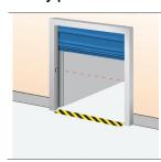
A set of a photocell transmitter with reflector or receiver is installed in the door opening. If the photocell beam is interrupted during closing, the door will stop in less than 30mm and reverse to the fully open position.
