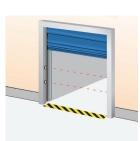
Two sets of photocell transmitters with reflectors and receivers are installed in the door opening. If one or both photocell beams are interrupted during closing, the door will stop in less than 30mm and reverse to the fully open position. Installed in the door opening.
