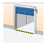
A pull rope switch next to the door opening can be operated from e.g. a forklift truck. Pulling the rope opens a closed door or closes an open door.
