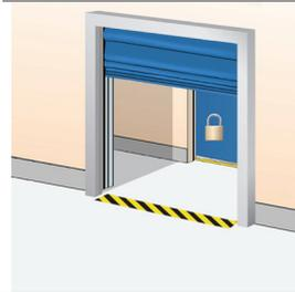
Developed for climate control or safety; if door A is open, door B cannot be opened. If door B is open; door A cannot be opened. Selector switch in control unit.
