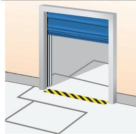
A sensor in the floor detects a metal object (usually forklift trucks, pallet trucks) and opens the door automatically. This is an ideal solution for frequent vehicle traffic.
