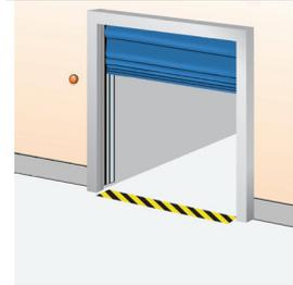
Flashing light during door movement.
