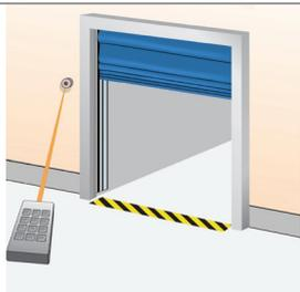
A hand-held radio transmitter allows door operation from a vehicle or any position within 50-100 meters from the receiver and aerial at the door.
