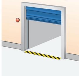
One or two red warning lights indicating that the door is moving or closed; continuous light when the door is closed, flashing light when the door is moving or not fully open.
